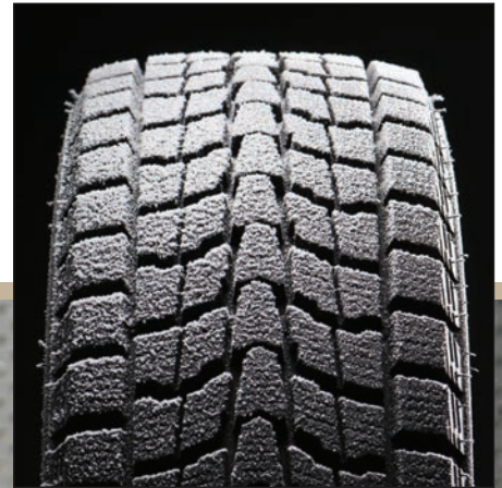
Fine-grade pumice is used as a tread enhancer for winter and all-weather tires to provide grip in snow and ice.
