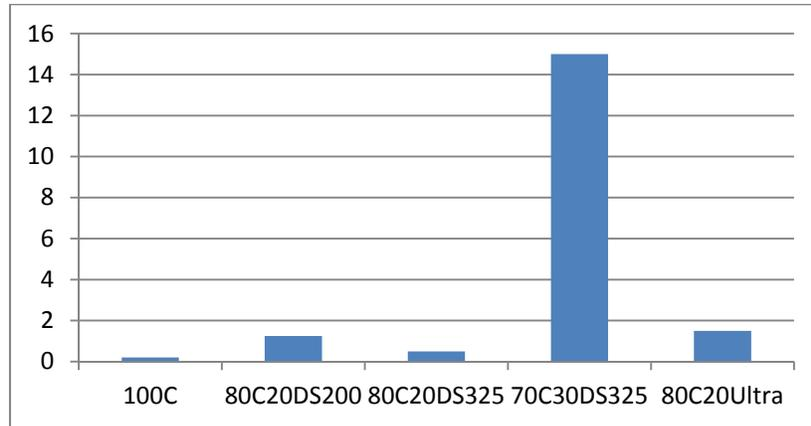
Fig. 7: Bleeding for different mixture designs
