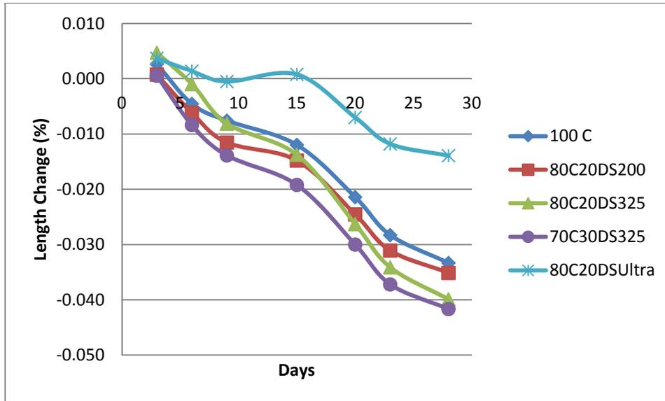
Fig. 13 Length Change (%) of Concrete Specimen due to shrinkage
