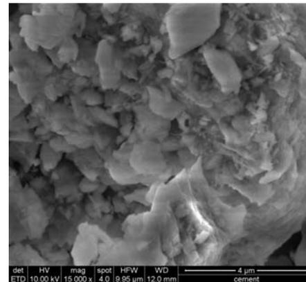
Fig. 2 Scanning Electron Micrograph for DS200 and Cement @ 2000X and 1500X
