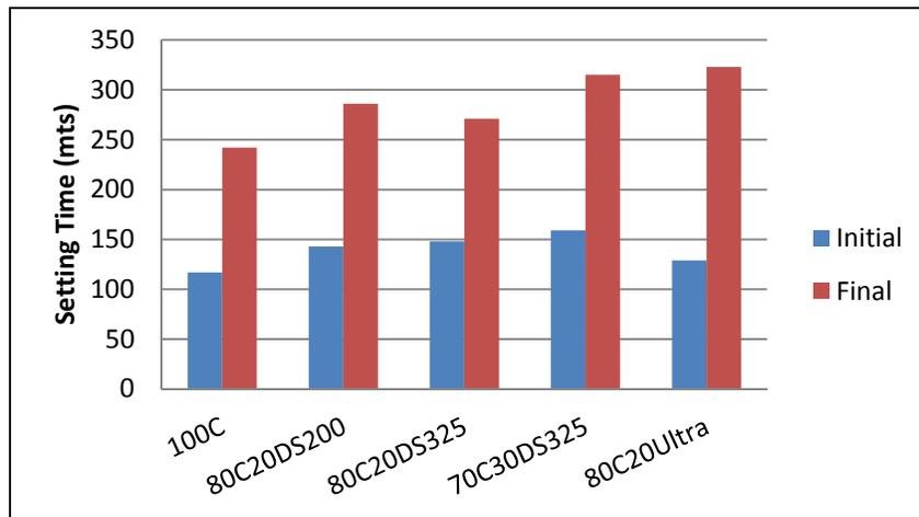
Fig. 8: Effect of Pumice on Setting Time
