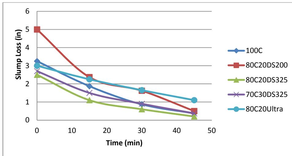
Fig. 6: Slump Loss versus Time Interval
