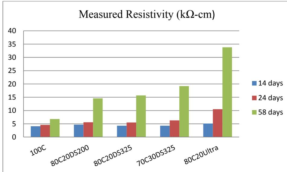
Fig. 12 Measured Resistivity of Concrete Specimens
