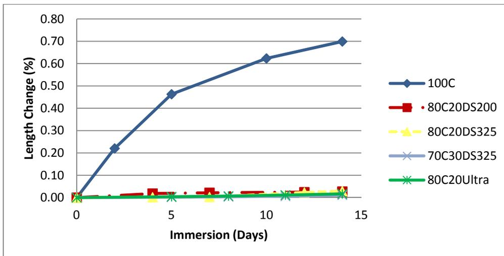
Fig. 14 Length Change (%) of Mortar Specimen due to ASR
