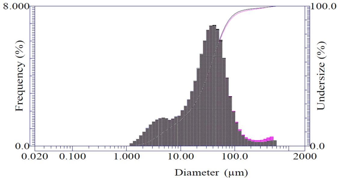
Fig. 3(c) Particle Size Distribution of “DS200” Pumice
