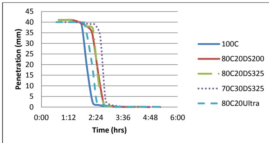
Fig. 9: Penetration resistance of different mixtures
