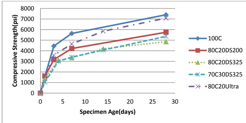
Fig. 10 Compressive strength for 4X8 cylinders
