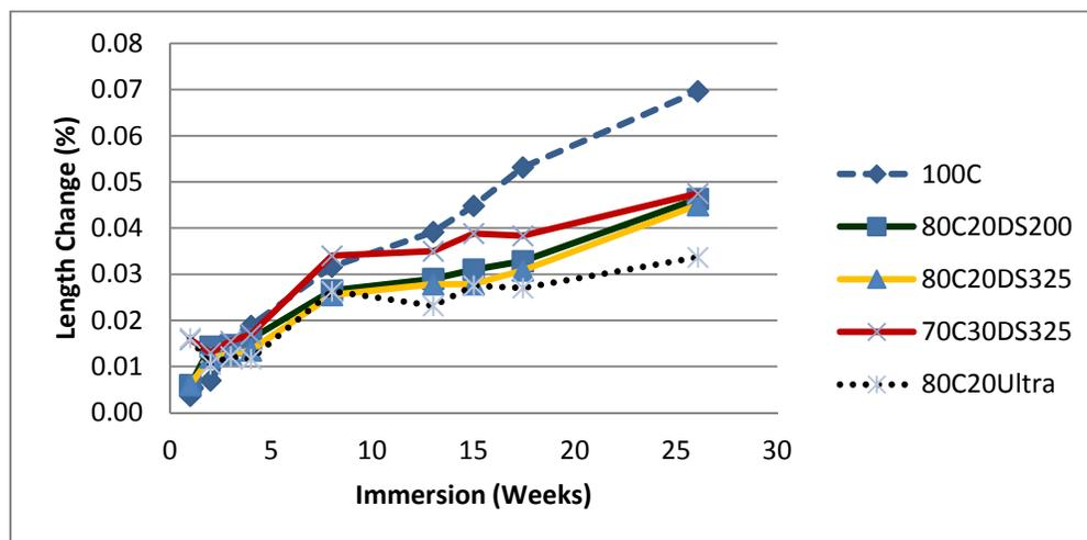
Fig. 11 Length Change (%) of Mortar Specimen due to sulfate
