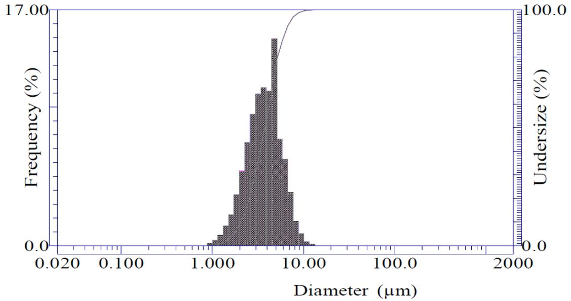
Fig. 3(a) Particle Size Distribution of "Ultrafine" Pumice
